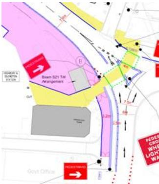
Water filled barrier location has caused limited width for the slip road off the gyratory. Vehicles observed to sit over the centre line (circled area) which is blocking traffic wishing to travel clockwise around the gyratory.
